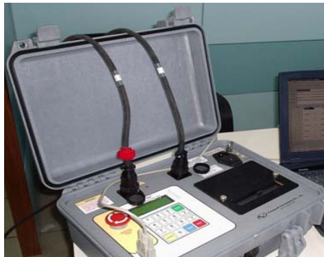
Figure 4.14: Transformer Turn Ratio Tester
