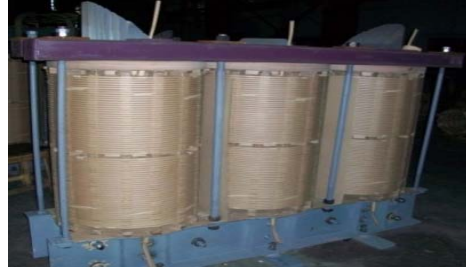
Figure 4.9(b): Core coil assembly completed
