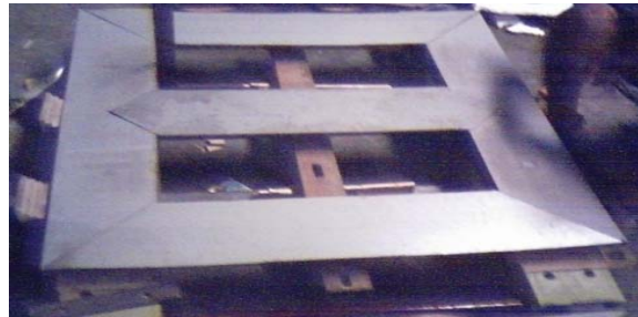
Figure 4.6(a):Core assembling at primary stage
